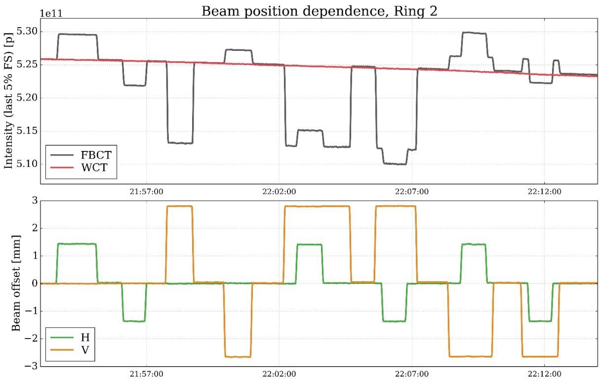
Figure 2: Comparison of beam position dependence for FBCT (black) and WCT (red) on Ring 2
